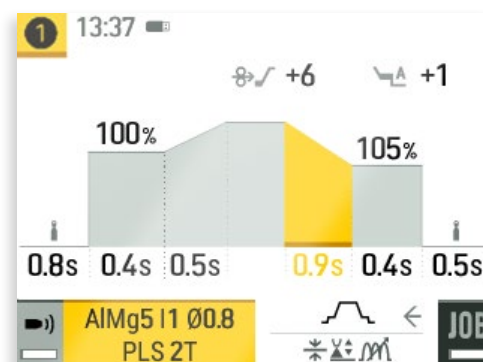
Settings: Pre-gas, Wire creep, Hot start, Upslope, Downslope, Crater fill, Burn back, Post-gas
