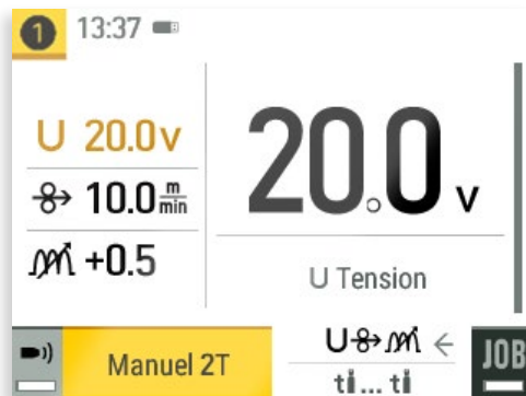
Settings: Voltage, Wire Speed and Inductance
